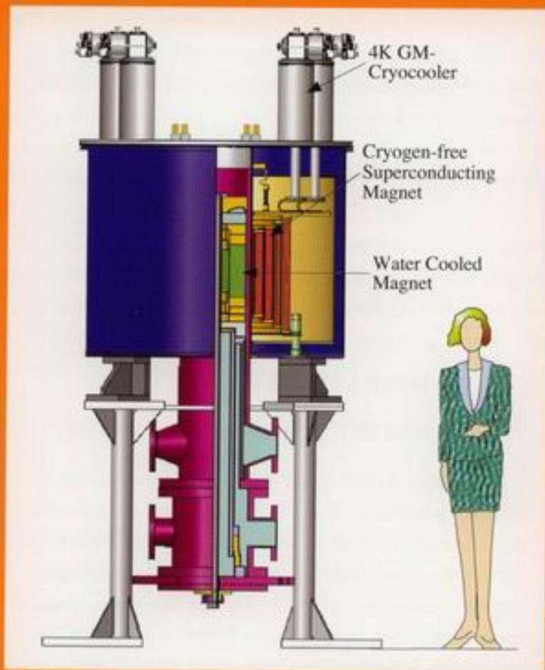
High Field Laboratory for Superconducting Materials,
