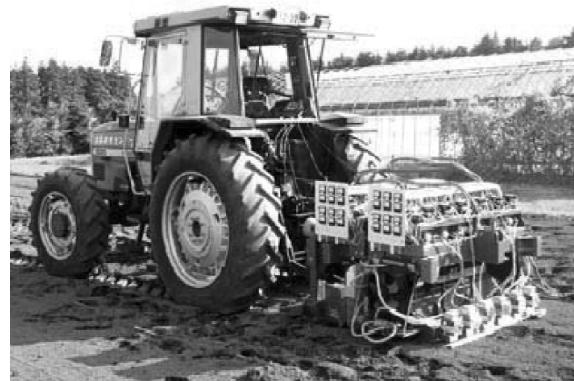
Fig. 4 Microwave soil disinfection tractor.
