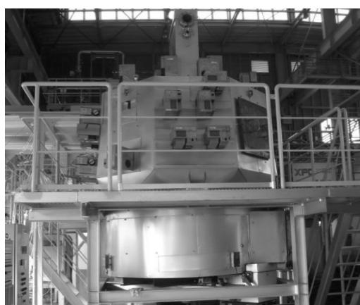
Fig. 5 Degradation furnace of dioxin in soil and fly ash by using microwave pyrolysis.
